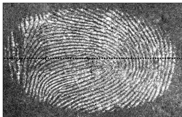
Figure 3. A fresh sebaceous fingerprint (after soaking in water for 5 min and drying under air) developed by treatment with 2 , followed by Ag-PD.
